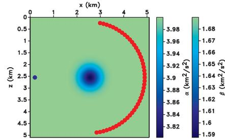
Figure 1: 2D synthetic  $\alpha$  and  $\beta$  models containing a negative Gaussian velocity anomaly with a constant background model. The acquisition geometry includes 20 shots, sampled every  $18^\circ$ , with 46 receivers for each shot. The source and receivers are on opposite sides of the anomaly in order to record waves transmitted through the anomaly.
