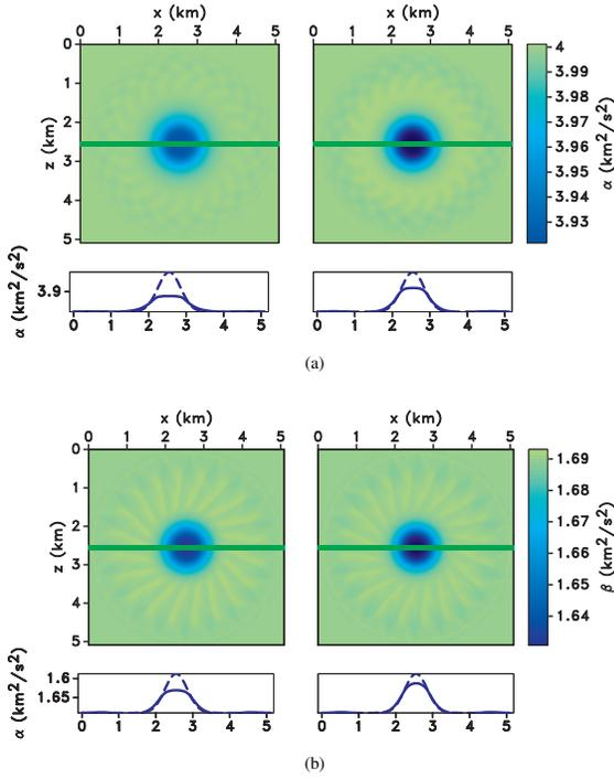
Figure 2: Updated (a)  $\alpha$  and (b)  $\beta$  models after 10 iterations, using objective function  $\mathcal{J}_D$  (left panels) and  $\mathcal{J}_D + \mathcal{J}_C$  (right panels). The bottom panels are subsets of the model at depth  $z = 2.55$  km. The solid and dashed lines are the updated and true models, respectively. The updated  $\alpha$  and  $\beta$  using objective function  $\mathcal{J}_D + \mathcal{J}_C$  is closer to the true model.
