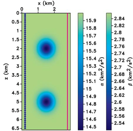
Figure 4: The  $\alpha$  and  $\beta$  models with two negative Gaussian anomalies. The dots are the source locations at  $x = 0.2$  km, and the vertical line shows the receivers at  $x = 2.8$  km.
