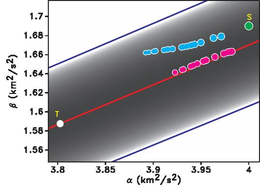
Figure 7: Model updates, as a function of iterations for the example in Figure 4. The dots represent the model at (1.5, 2) km. The red and blue dots are the updated models with and without constraints, respectively. Using the constraints forces the  $\alpha$  and  $\beta$  models closer to the true model.
