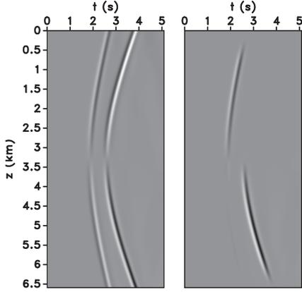
Figure 5: Left panel: the horizontal component of a shot gather with the source at  $z = 3.5$  km. The early arrival is the P-wave and later arrival is the S-wave. Right panel: the processed data for inversion with P-waves only from  $z = 0$  to 3.5 km and S-waves only from  $z = 3.5$  to 7 km.
