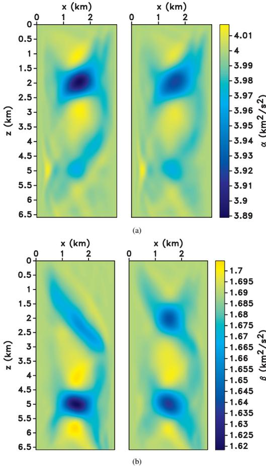
Figure 6: Updated (a)  $\alpha$  and (b)  $\beta$  models after 21 iterations, using objective function  $\mathcal{J}_D$  (left panels) and  $\mathcal{J}_D + \mathcal{J}_C$  (right panels). Note that the Gaussian anomaly at (1.5, 2) km is better recovered in right panel of (b).
