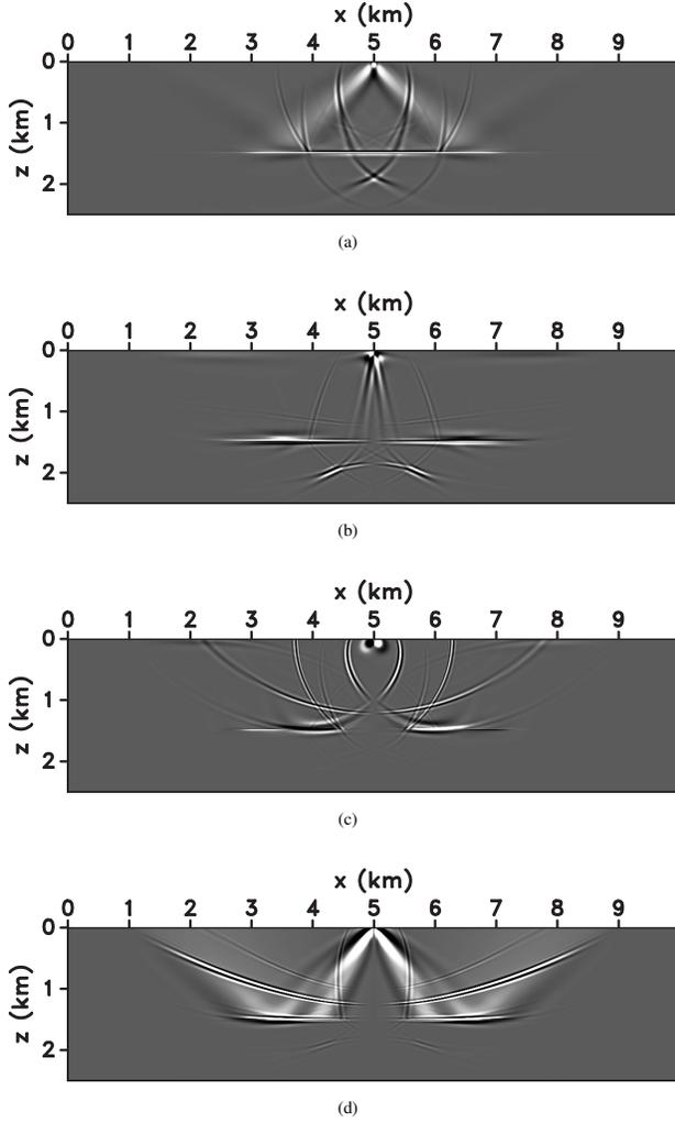
Figure 1: Images with scalar and vector potentials: (a) PP, (b) PS, (c) SP and (d) SS. Note that backscattering artifacts do not occur in (b) and (c) due to correlation of different wave modes.
