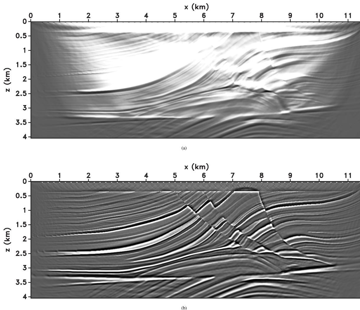
Figure 3: Marmousi elastic migration with the energy imaging condition. Energy image using (a) imaging condition equation 15, and (b) imaging condition equation 25. The image in (b) shows no artifacts from polarity reversal and attenuated backscattering energy compared to (a).
