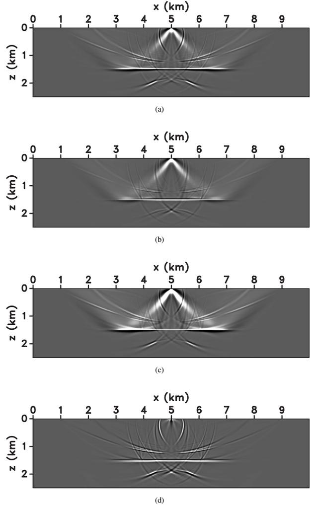
Figure 2: (a) Kinetic and (b) potential energy images; total energy image (c) with and (d) without backscattering.
